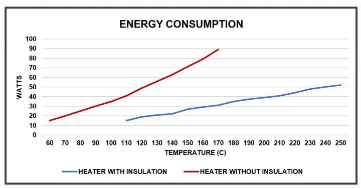
In house testing has shown that using insulation alongside our silicone heaters offers an average energy saving of 63%.
