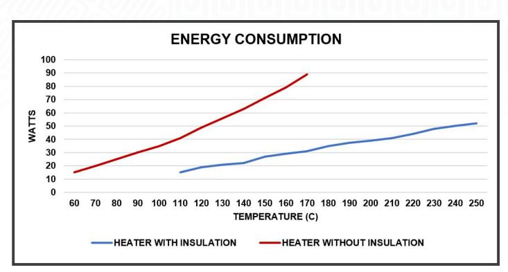
In house testing has shown that using insulation alongside our silicone heaters offers an average energy saving of 63%.
